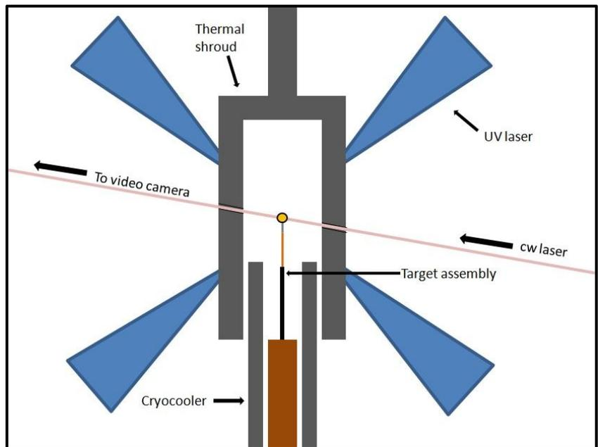
**Fig. 1 The geometry of the OMEGA target chamber**
