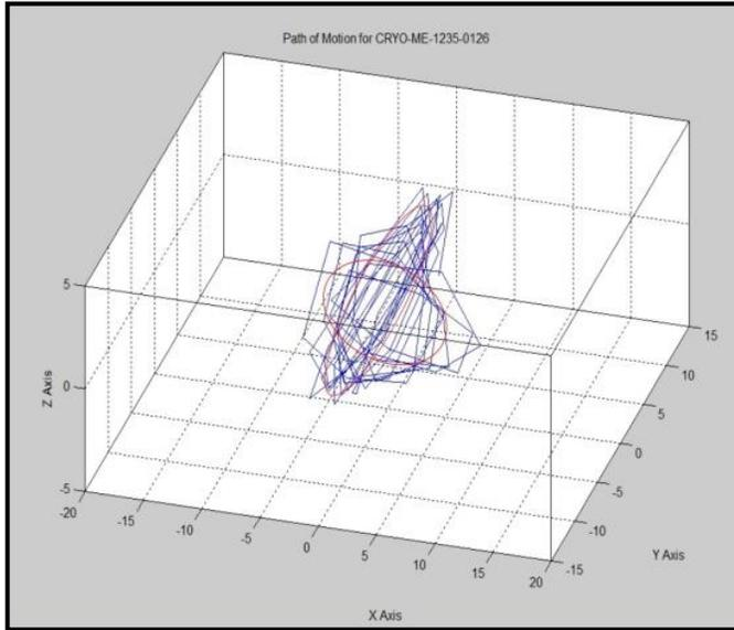
**Fig. 10 Degeneration of distinct elliptical motion path around a threshold frequency of 300 Hz**
