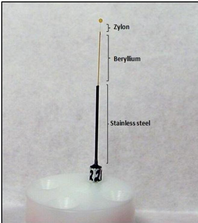
**Fig. 2 Anatomy of a Type 1 mass equivalent fusion target**
