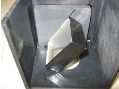
Figure 3: apparatus used to hold Brewster's angle polarizer
