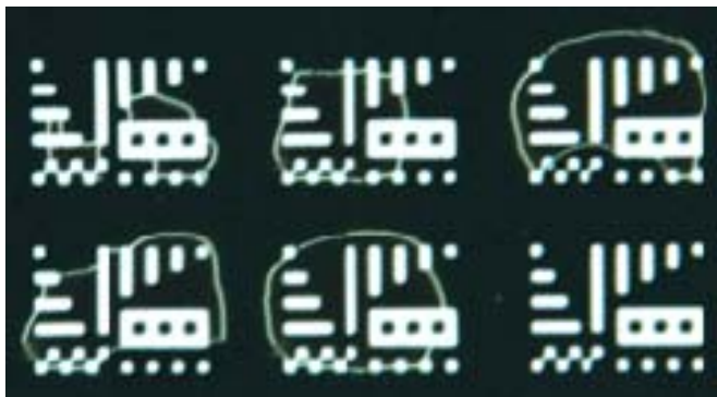
Figure 6: domains of reverse twist
