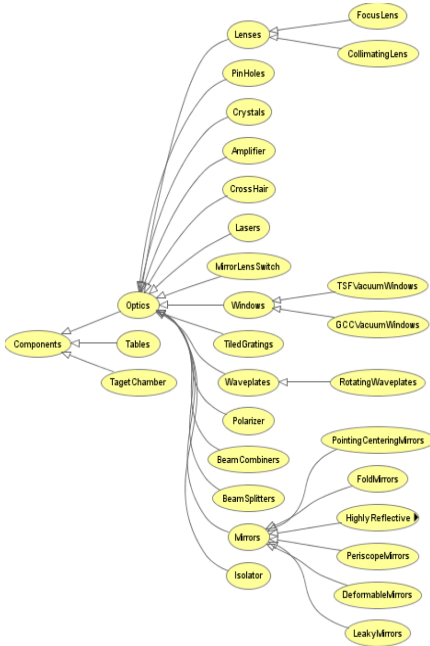
Figure 1. A portion of the class structure for LLE's Ontology, each line representing an "is a" relationship.
