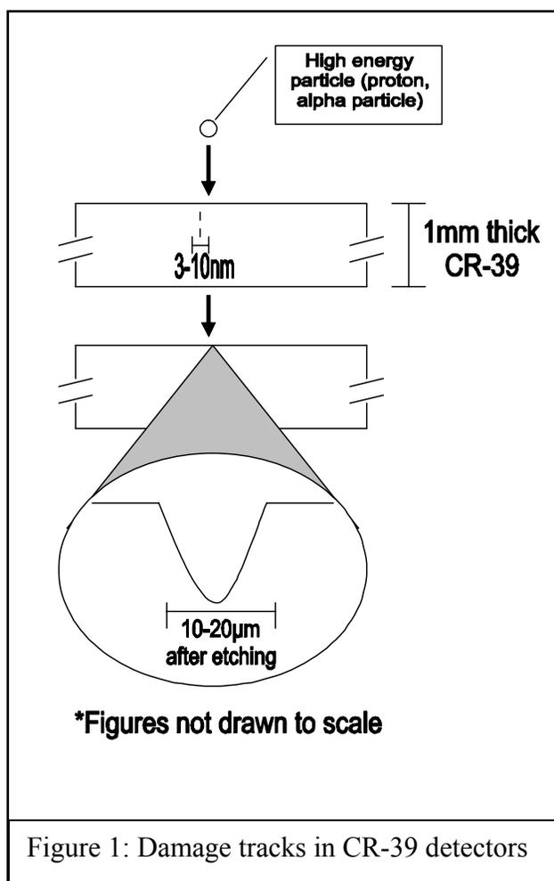
Figure 1. These pits, about 10-20  $\mu$ m in diameter, are visible under a digital microscope. The etched tracks can thus be examined using the Charged Particle Spectroscopy (CPS) program developed by scientists at MIT.
