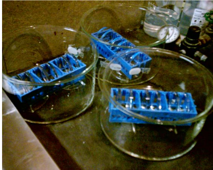
Figure 2: Sealed containers where various coated substrates were exposed to contaminants.
