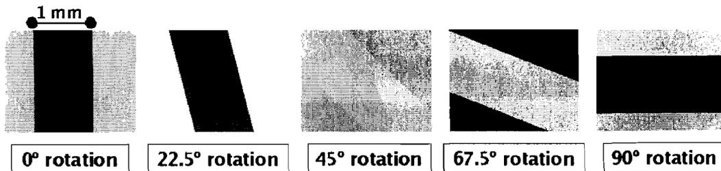
Figure 5: 2-domain cell rotated under crossed polarizers to show contrast.
