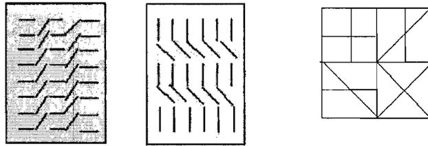
*Figure 6: At left, diagrams of alignment directions on the two substrates of a 4-domain cell. At right is a diagram of the twist created in the pattern of four repeating alignment domains when the cell is assembled with the two substrates shown at left: clockwise from top left, 90°, 45°, 90°, and 45° of twist are visible.*
