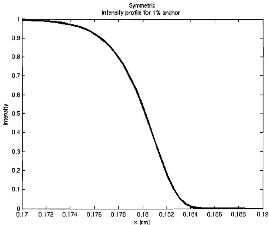
Fig. 4 – *In the symmetric beam edge, both the upper portion and lower portion have the same super Gaussian order.*
