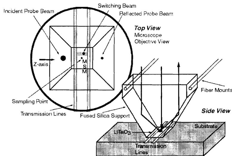
The diagram in Fig. 3.2 is a representation of the finger probe. A finger probe consists of an EO crystal with a fused silica support mounted to it in such a way that the angles of the support can provide total internal reflection for the probe beam entering the
