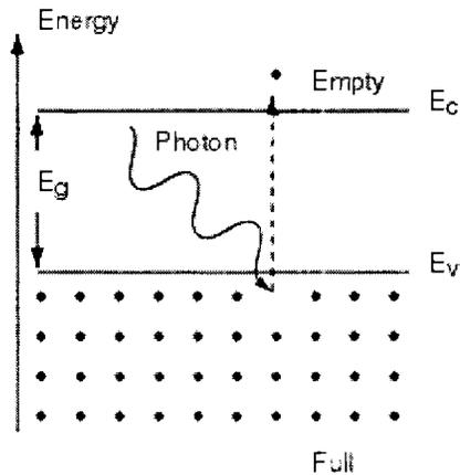
Absorption of photons with energy greater than that of the band gap results in generation of excited electrons that are now free to flow in the conduction band. These conditions allow a semiconductor to exhibit conductive properties when excited by light of the wavelength  $> E_g$ .
