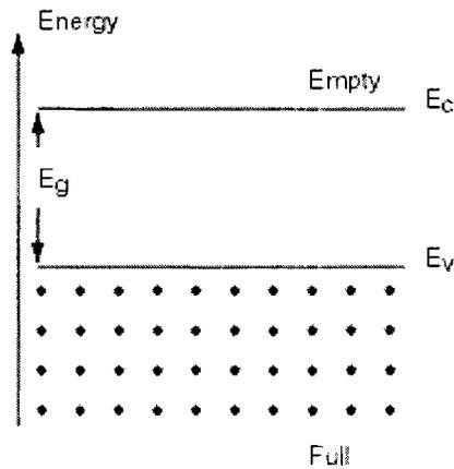
The energy-band diagram shows the conduction-band edge ( $E_c$ ) above which all states are empty, the valence-band edge ( $E_v$ ) below which all states are occupied by electrons. The energy difference between ( $E_c$ ) and ( $E_v$ ) is the band gap energy ( $E_g$ ). The following diagram (figure 2.2) represents the same semiconductor exposed to light with photon energy ( $h\nu$ ) at least equal to  $E_g$ .
