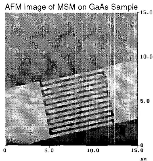
MSM structures have been fabricated with finger spacing and width as small as 100 nm on low-temperature grown GaAs. The particular samples of MSM GaAs samples used in this study were of ~300 nm finger width and ~200 nm spacing.
