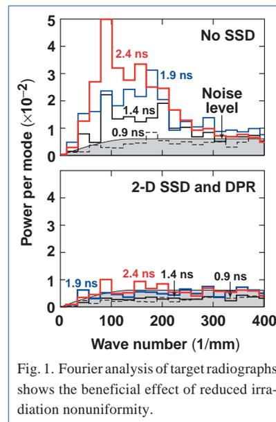
Fig. 1. Fourier analysis of target radiographs shows the beneficial effect of reduced irradiation nonuniformity.
