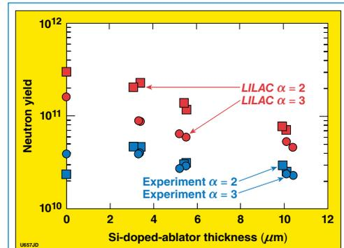
Figure 1. Calculated and measured neutron yields for the Si-doped-ablator implosions plotted as a function of the thickness of the Si-doped ablator. Red points are predictions from the 1-D hydrodynamics code *LILAC*. Blue points are the experimental measurements. The squares are for the  $\alpha = 2$  pulse shape and the circles are for the  $\alpha = 3$  pulse shape.
