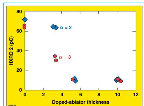
Figure 2. The intensity of x rays with an energy  $>50$  keV is plotted as a function of the thickness of the Si-doped ablator. The diamond points are for the  $\alpha = 2$  pulse shape and the circles are for the  $\alpha = 3$  pulse shape.
