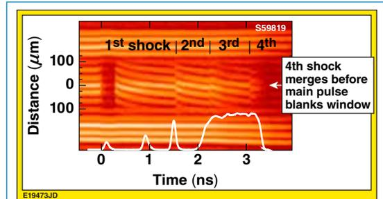
Figure 2. VISAR shock data for an experiment where the driving laser pulse (shown on the bottom of the figure) consisted of three short pulses followed by a high-energy long pulse. This pulse configuration generates four shocks that merge at ~3.1 ns.
