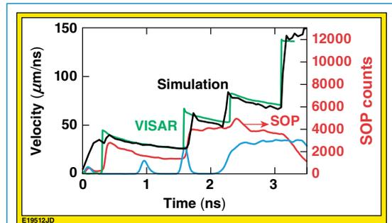
Figure 3. Green curve: shock velocities inferred from streak camera data of Fig. 2; red curve: SOP signal (arbitrary units) and blue curve: laser pulse time history (arbitrary units); black curve, theoretical simulation.
