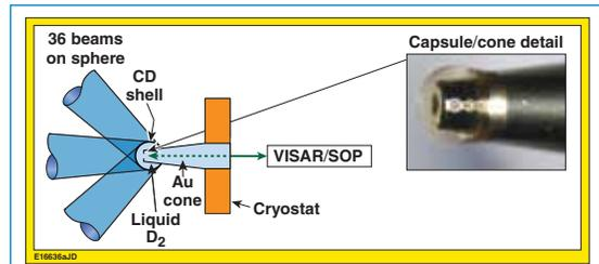
Figure 1. Schematic (left) and photograph of cone-in-shell target used to conduct multiple shock-timing tests on the OMEGA laser.
