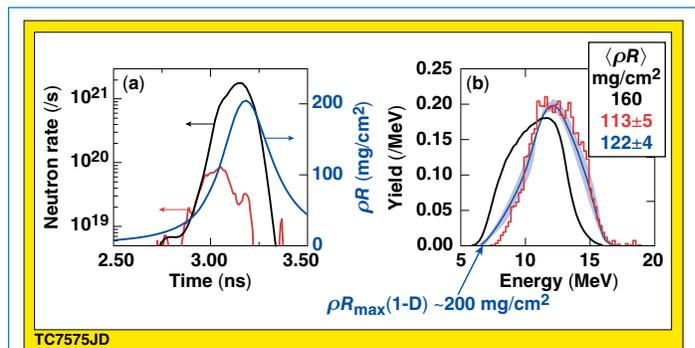
Figure 2. The same plots as Fig. 1 for a low-adiabat implosion ( $\alpha \sim 2$ ) of a 27- $\mu\text{m}$ -thick CH shell with 15 atm  $\text{D}_2$ . The difference in the spectra at the low-energy tail corresponds to  $\sim 15\%$  reduction in the peak value of the measured areal density compared to the simulated value.
