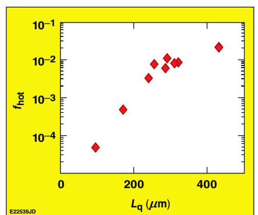
Figure 3. The fraction of laser energy converted to hot electrons at an intensity of  $7 \times 10^{14}$  W/cm<sup>2</sup> was measured using the hard x-ray diagnostic.
