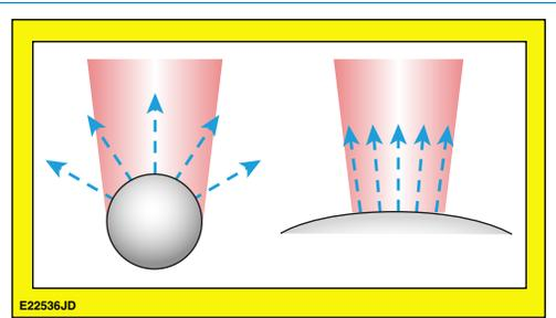
Figure 1. A schematic illustrating the scale length control in this experiment. As the radius of the target decreases, the plasma expansion becomes more divergent and shorter density scale lengths are produced at the quarter-critical surface.
