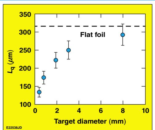
Figure 2. The density scale length at a density of  $10^{21}$  cm<sup>-3</sup> was measured using the angular filter refractometer.
