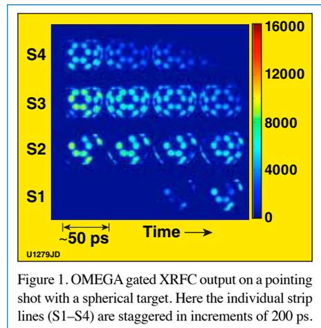
Figure 1. OMEGA gated XRFC output on a pointing shot with a spherical target. Here the individual strip lines (S1–S4) are staggered in increments of 200 ps.
