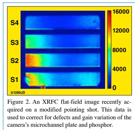
Figure 2. An XRFC flat-field image recently acquired on a modified pointing shot. This data is used to correct for defects and gain variation of the camera’s microchannel plate and phosphor.
