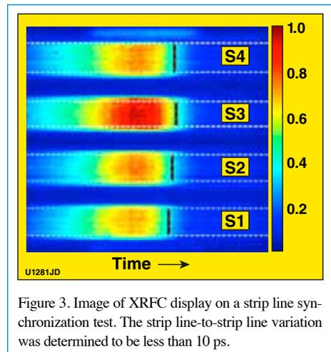
Figure 3. Image of XRFC display on a strip line synchronization test. The strip line-to-strip line variation was determined to be less than 10 ps.
