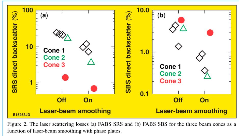
Figure 2. The laser scattering losses (a) FABS SRS and (b) FABS SBS for the three beam cones as a function of laser-beam smoothing with phase plates.
