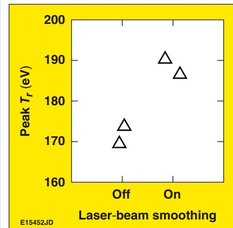
Figure 1. The peak radiation temperature inferred from the x-ray flux levels measured with the DANTE diagnostic as a function of laser-beam smoothing with phase plates.
