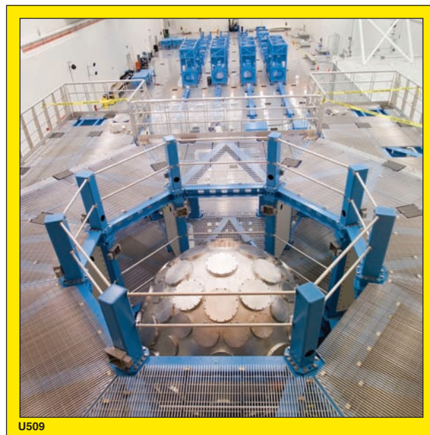
Figure 2. View of the OMEGA target chamber nested within the target-area structure.
