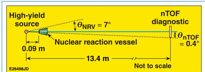
Figure 1. Schematic of a nuclear science experiment on the OMEGA laser.
