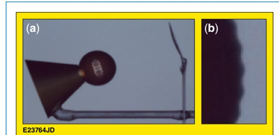
Figure 1. Photograph of a cone-in-shell target for studies of hydrodynamic instability growth in spherical, direct-drive geometry on the NIF. The target comprises a plastic capsule, a gold cone, and a backlighter. (b) Single-mode perturbations are machined onto the capsule surface to act as instability seeds.
