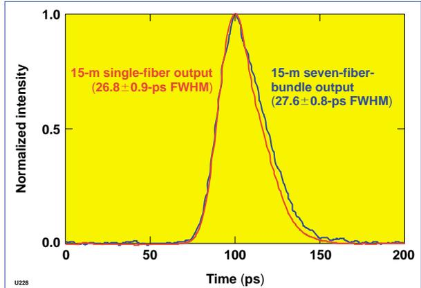
Figure 1. Comparison of short-pulse propagation through single- and seven-fiber bundle.
