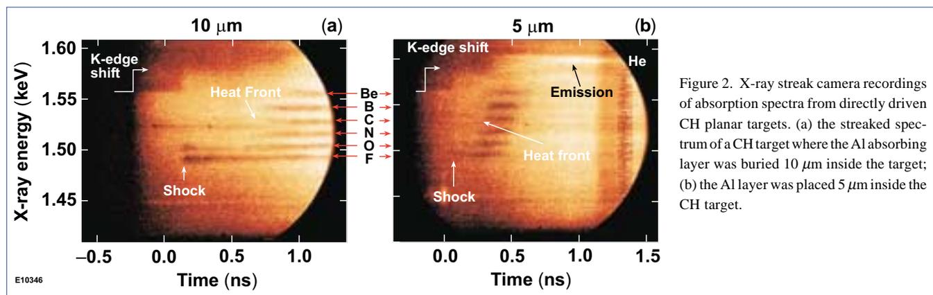
Figure 2. X-ray streak camera recordings of absorption spectra from directly driven CH planar targets. (a) the streaked spectrum of a CH target where the Al absorbing layer was buried 10  $\mu$ m inside the target; (b) the Al layer was placed 5  $\mu$ m inside the CH target.
