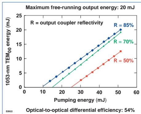
Fig. 2. Free-running output of laser versus pumping energy.
