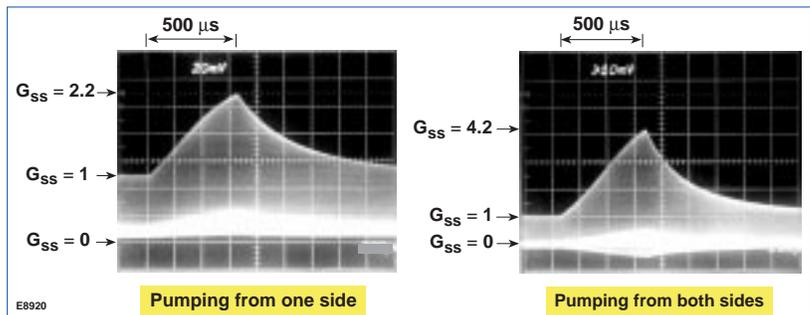
Fig. 1. Measurement of small-signal gain of diode-pumped amplifier for one-sided pumping (left) and two-sided pumping (right).
