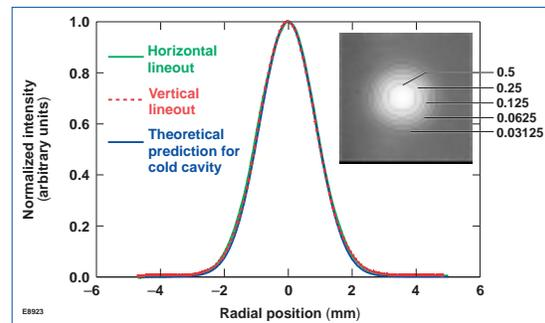
Fig. 3. Output beam profile at 6.4-mJ output energy. Insert is the image of the laser beam on the logarithmic scale with superimposed contour lines.
