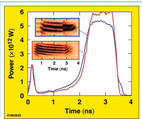
Figure 3. Pulse shape and VISAR fringe records from shot 50548.
