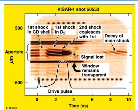
Figure 2. VISAR fringe record and laser pulse shape of shot 50553.
