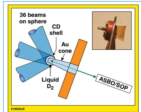
Figure 1. Schematic of experimental configuration and photograph of target (inset).
