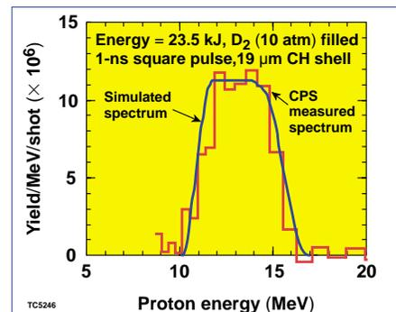
Figure 3. Secondary proton spectra from OMEGA shots 17663, 17664, 17665, and 17669 combined (red line). The blue line is the simulated spectrum for a capsule areal density of  $\sim 50 \text{ mg}/\text{cm}^2$  and the CPS setup parameters.
