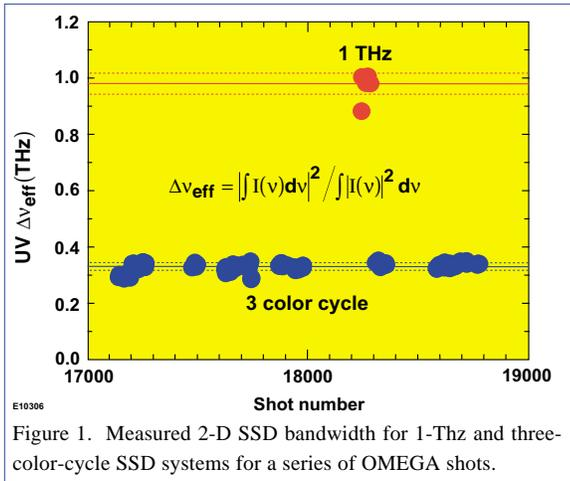
Figure 1. Measured 2-D SSD bandwidth for 1-THz and three-color-cycle SSD systems for a series of OMEGA shots.
