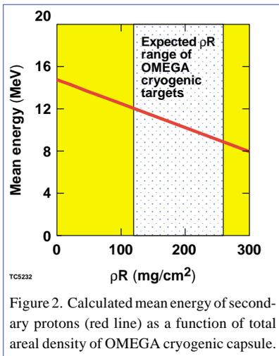
Figure 2. Calculated mean energy of secondary protons (red line) as a function of total areal density of OMEGA cryogenic capsule.
