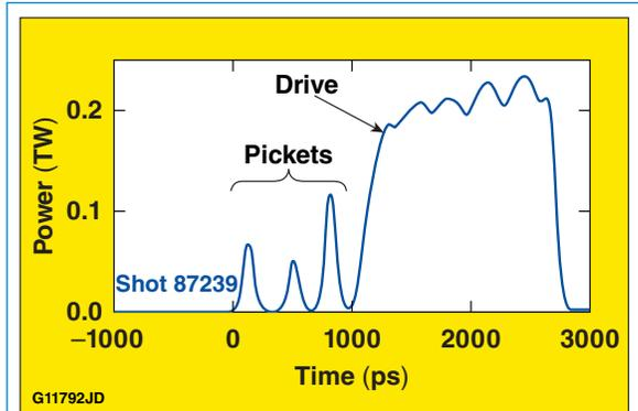
Figure 1. Typical cryogenic-implosion pulse shape. The pulse is typically divided into one or more “features,” 1 to 3 “pickets” preceding the main “drive.”
