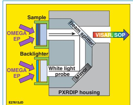
Figure 1. Schematic of the targets and optical train used in this experiment. UV beams drive the target packages mounted on the front of a powder x-ray diffraction image-plate (PXRDIP) box. White light from the backlighter is directed to the back surface of the aluminum sample via a titanium mirror and 50R/50T beam splitter. Additionally, this geometry allows the VISAR laser to probe the Al–LiF interface during exposure to the white light.
