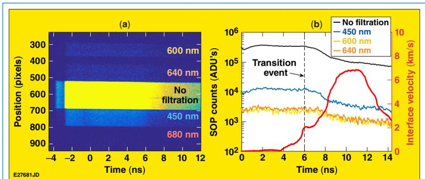
Figure 2: OMEGA EP shot 28400. (a) SOP streak image with filtered regions indicated by their filter's central wavelength. The region with no filtration is used to compare with undriven reference shots. (b) Lineouts of the SOP streak record overlaid with the Al–LiF interface velocity extracted from VISAR. A drop in the reflected probe's intensity, beginning at 6 ns, occurs when the pressure at the Al–LiF interface reaches 30 GPa.
