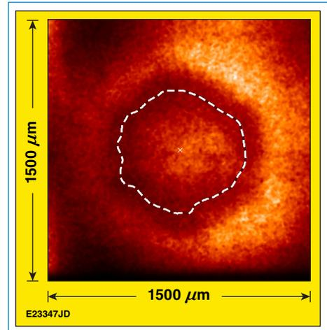
Figure 2. Images from backlit implosion N140612-001, using an Fe backlighter at a convergence ratio of ~2.8. The dashed line is the location of the surface of peak x-ray absorption.
