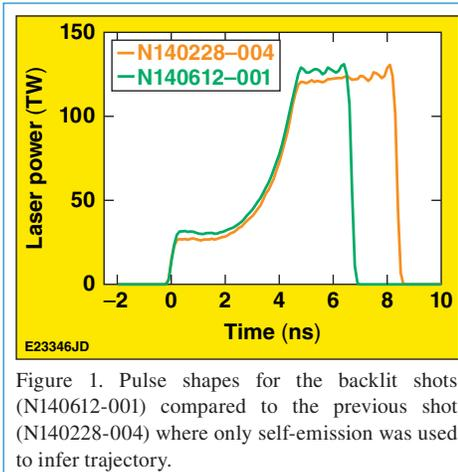
Figure 1. Pulse shapes for the backlit shots (N140612-001) compared to the previous shot (N140228-004) where only self-emission was used to infer trajectory.
