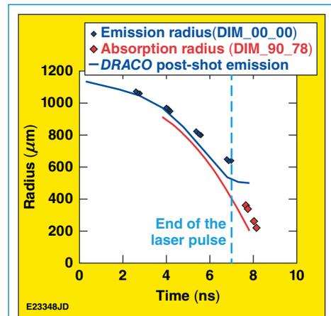
Figure 3. Trajectories inferred from self-emission images viewed from the pole compared to that inferred from backlit image viewed from the equator for NIF target shot N140612-001.
