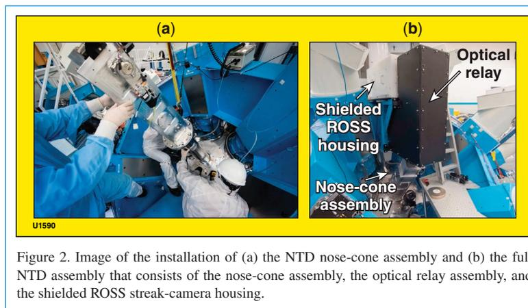
Figure 2. Image of the installation of (a) the NTD nose-cone assembly and (b) the full NTD assembly that consists of the nose-cone assembly, the optical relay assembly, and the shielded ROSS streak-camera housing.
