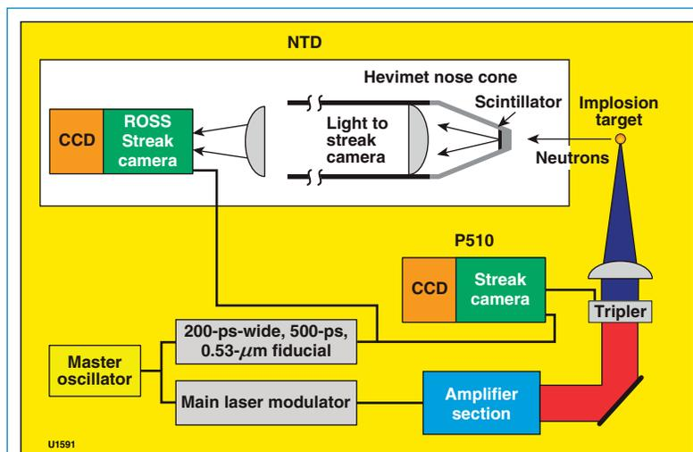
Figure 1. Setup of the neutron temporal diagnostic (NTD). CCD: charge-coupled device; P510: P510PSU streak tube.<sup>1</sup>
