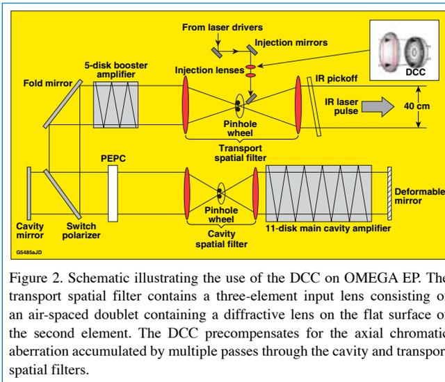
Figure 2. Schematic illustrating the use of the DCC on OMEGA EP. The transport spatial filter contains a three-element input lens consisting of an air-spaced doublet containing a diffractive lens on the flat surface of the second element. The DCC precompensates for the axial chromatic aberration accumulated by multiple passes through the cavity and transport spatial filters.
