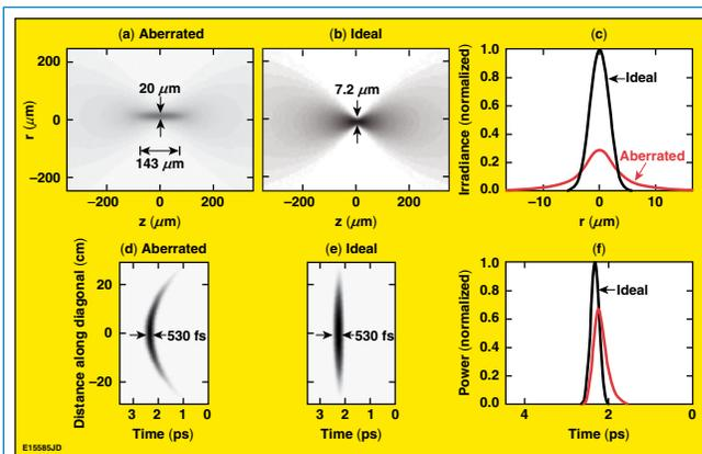
Figure 1. Modeling of the chromatic-aberration-induced fluence reduction [(a) to (c)] and pulse broadening [(d) to (f)] for OMEGA EP. The DCC simultaneously removes spatial and temporal distortions by compensation with negative dispersion.
