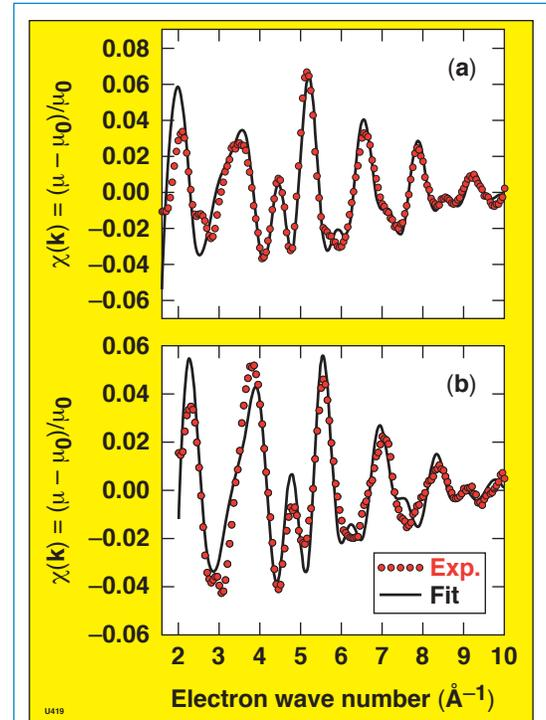
Figure 1. Fitting the measured V EXAFS spectra for the unshocked case (a) and the shocked case (b) with the FEFF8 code, which allows for multiple electron scattering. The fitting yields the temperature and compression of the shocked vanadium.
