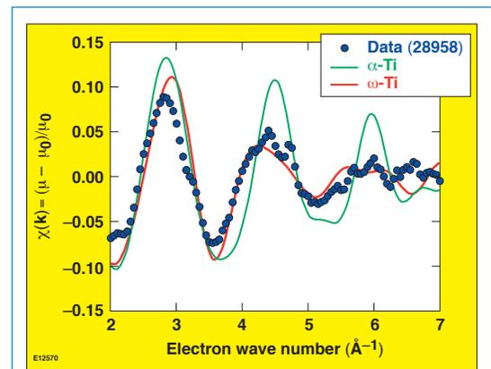
Figure 2. Fitting the FEFF8 EXAFS code to the measured Ti EXAFS spectrum assuming the  $\alpha$ -Ti phase (the hcp phase at normal conditions) and the  $\omega$ -Ti phase. Only the compression was adjusted (to fit the modulation frequency) and the LASNEX-predicted temperature  $T = 900$  K was assumed. A phase transformation  $\alpha$ -Ti $\rightarrow\omega$ -Ti is clearly indicated by the data.
