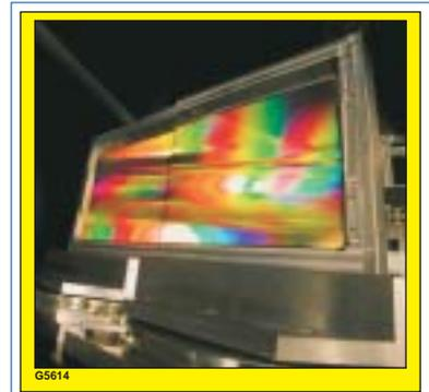
Figure 1. Photograph of tiled grating assembly. The gratings are artificially illuminated by an external light source.
