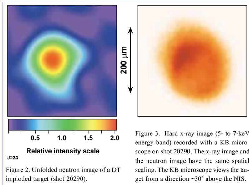
Figure 3. Hard x-ray image (5- to 7-keV energy band) recorded with a KB microscope on shot 20290. The x-ray image and the neutron image have the same spatial scaling. The KB microscope views the target from a direction  $\sim 30^\circ$  above the NIS.
