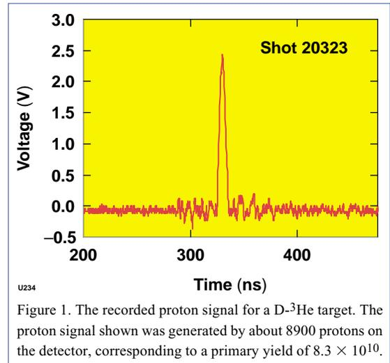
Figure 1. The recorded proton signal for a D- $^3\text{He}$  target. The proton signal shown was generated by about 8900 protons on the detector, corresponding to a primary yield of  $8.3 \times 10^{10}$ .
