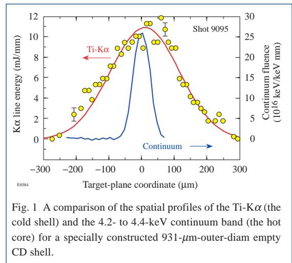
Fig. 1 A comparison of the spatial profiles of the Ti- $K\alpha$  (the cold shell) and the 4.2- to 4.4-keV continuum band (the hot core) for a specially constructed 931- $\mu\text{m}$ -outer-diam empty CD shell.
