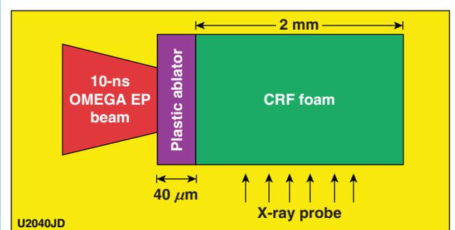
Figure 1. Schematic of the foam package and geometry of experiment. One beam (from the left) drives a shock wave into the carbonized resorcinol foam with a density of 0.1 g/cm<sup>3</sup>. The remaining three beams generate an x-ray probe beam that penetrates the shocked foam. The imaging x-ray Thomson spectrometer diagnostic records the scattered x-ray spectrum spatially resolved along the axis of the foam.
