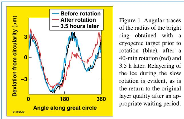
Figure 1. Angular traces of the radius of the bright ring obtained with a cryogenic target prior to rotation (blue), after a 40-min rotation (red) and 3.5 h later. Relayering of the ice during the slow rotation is evident, as is the return to the original layer quality after an appropriate waiting period.
