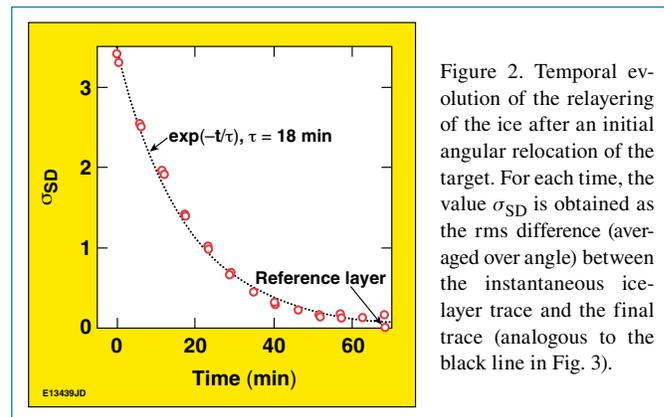
Figure 2. Temporal evolution of the relayering of the ice after an initial angular relocation of the target. For each time, the value  $\sigma_{SD}$  is obtained as the rms difference (averaged over angle) between the instantaneous ice-layer trace and the final trace (analogous to the black line in Fig. 3).
