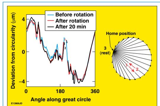
Figure 3. Improved shadowgraphic image acquisition method that avoids relayering through short excursions to the desired angular position followed by a return to the “home” position. The resulting bright ring traces before and after the angular excursion as well as 20 min later show no evidence of relayering (a). The scan pattern for acquiring the data is shown in (b).
