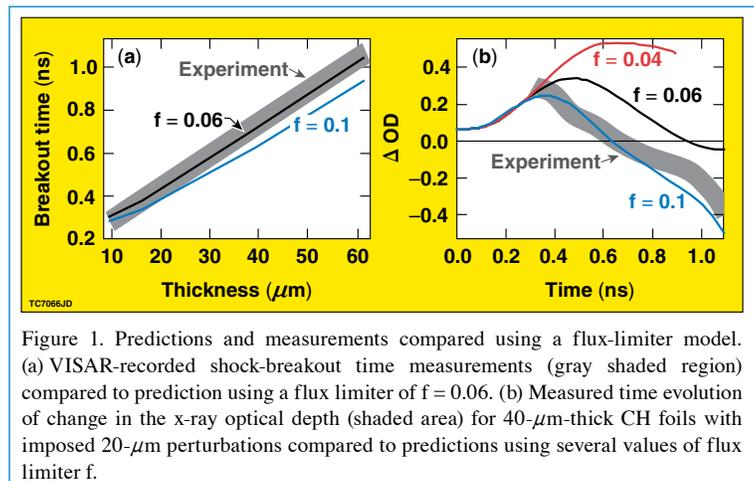
Figure 1. Predictions and measurements compared using a flux-limiter model. (a) VISAR-recorded shock-breakout time measurements (gray shaded region) compared to prediction using a flux limiter of  $f = 0.06$ . (b) Measured time evolution of change in the x-ray optical depth (shaded area) for 40- $\mu$ m-thick CH foils with imposed 20- $\mu$ m perturbations compared to predictions using several values of flux limiter  $f$ .
