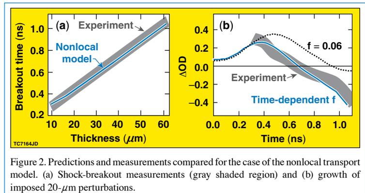
Figure 2. Predictions and measurements compared for the case of the nonlocal transport model. (a) Shock-breakout measurements (gray shaded region) and (b) growth of imposed 20- $\mu$ m perturbations.
