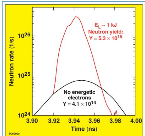
Figure 2. The neutron yield increases by more than an order of magnitude when a properly timed, high-energy electron source irradiates the compressed capsule.
