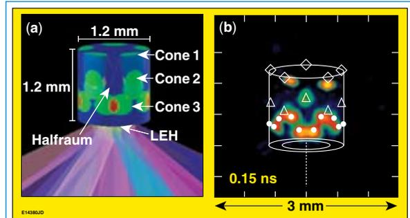
Figure 1. (a) VISRAD model of an empty scale-3/4 Au halfraum being irradiated with 20 laser beams that are smoothed with elliptical phase plates and arranged in 3 cones. (b) A gated ( $\Delta t = 80 \text{ ps}$ ) hard x-ray ( $>8 \text{ keV}$ ) image generated at  $t = 0.15 \text{ ns}$  as the laser beams strike the inner wall of the halfraum. The plotting symbols represent the locations of the centers of the cone-1 beams (diamonds), cone-2 beams (triangles), and cone-3 beams (circles).
