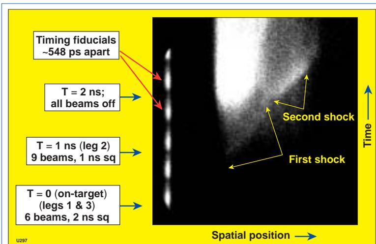
Figure 2. SOP data for a Be wedge experiment on OMEGA shot 25964. The narrow side of the wedge is on the left. The SOP image shows the first shock merging with the second shock near the center of the image. The target and hohlraum drive were designed to provide shock coalescence near the center of the SOP image.
