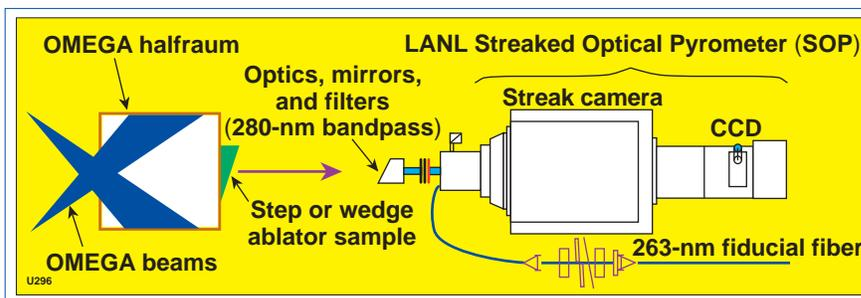
Figure 1. Schematic of shock propagation experiments. An ablator sample in the form of a wedge is placed on the back of a half-hohlraum cylinder (halfraum). The SOP resolves the shock breakout signature along the wedge. UV (263-nm)-laser, 100-ps pulses are used as a timing fiducial.
