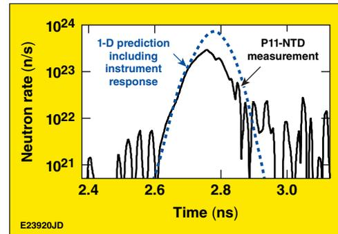
Figure 1. Measured neutron production rate (solid line) from the P11-NTD detector for a layered cryogenic DT target (shot 76607) with a yield of  $3.5 \times 10^{13}$  compared with 1-D predictions (dashed line).
