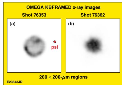
Figure 2. X-ray images obtained with the new OMEGA diagnostic KBFRAMED. (a) Image at peak stagnation of a  $\text{D}_2$ -filled CD shell. (b) Image at peak stagnation of a cryogenic DT target. The approximate point-spread function (psf) is indicated.
