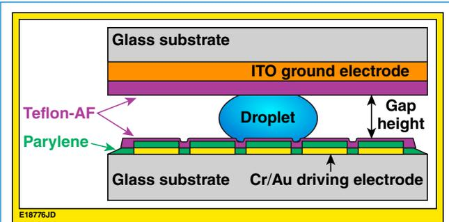
Figure 1. The patterned glass structure used to dispense and move droplets of oil and water is shown in cross-section.
