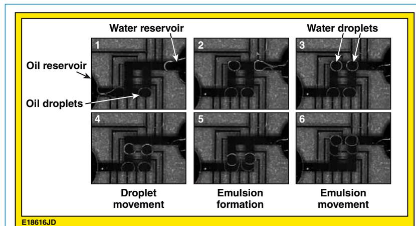
Figure 2. Time-lapse images show the formation of droplets of oil and water from two reservoirs (1–3); movement of the droplets (4); combination of the droplets to form an emulsion (5), and, finally, movement of the emulsion.
