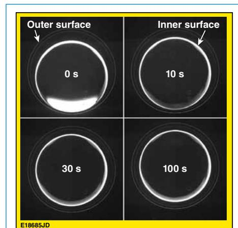
Figure 3. Time-lapse images of an oil-in-water emulsion suspended in oil is shown in a dark field image. The inner and outer surfaces are defined by the bright rings. The buoyancy mismatch has the oil droplet initially at the bottom of the water droplet and supported by surface tension. Applying an electric field ( $10^4$  V/m) centers the two droplets within 100 s.
