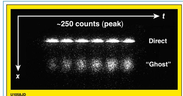
Figure 3. The UV fiducial comb pulse delivered to a prototypical x-ray fiducial streak camera with a prototypical UV fiber link produces a high-contrast fiducial mark with good signal to noise (direct).
