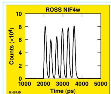
Figure 2. The UV fiducial comb pulse measured with a ROSS streak camera meets the NIF $4\omega$ Fidu requirements.
