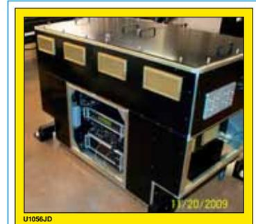
Figure 1. The NIF $4\omega$ Fidu laser system is built in a portable workstation in the NIF target bay so that it can be removed easily for high-yield target shots. The enclosure serves as both a laser safety barrier and provides EMI protection to the laser and electronics during target shots.
