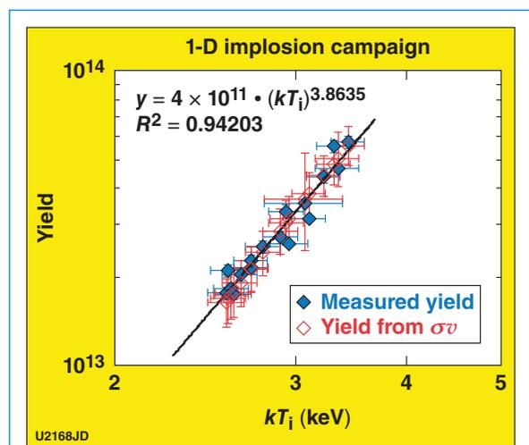
Figure 2. Neutron yield plotted versus the minimum ion temperature taken from the nTOF measurements. The data are shown as filled diamonds with measurement error bars. The open diamonds are yields calculated from the reactivity ( $\sigma v$ ) temperature dependence.
