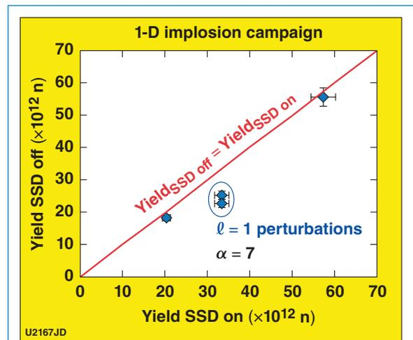
Figure 1. Plot of neutron yield with SSD off versus neutron yield with SSD on. Data are shown as diamonds with errors. The line represents the condition where the SSD-off yield is the same as the SSD-on yield. Circled points are implosions with an initial  $\ell = 1$  perturbation.
