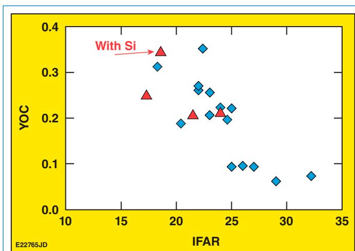
Figure 1. The yield ratio with 1-D prediction [yield over clean (YOC)] is plotted as a function of the calculated in-flight aspect ratio (IFAR) for triple-picket cryogenic DT implosions in 2013. The red triangles are the Si-coated CD shells, which perform similarly to uncoated CD shells (blue diamonds). This suggests that shinethrough is not the dominant source for hydro-instability seeds.
