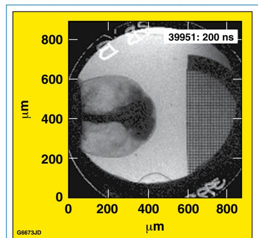
Figure 2. X-ray radiograph from an NLUF experiment that simulates astrophysical jets by driving a high-density jet into a foam.
