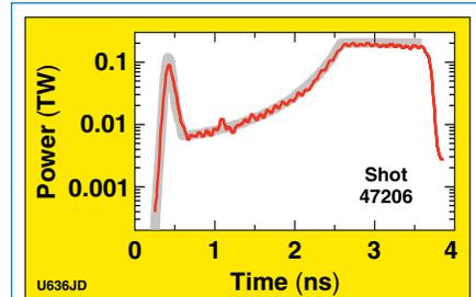
Figure 1. The drive pulse used to achieve a neutron-averaged areal density of  $202 \pm 7 \text{ mg/cm}^2$  on shot 47206. The pulse (red curve) matches closely with the design specifications (the thickness of the gray curve represents the design tolerances on the drive pulse).
