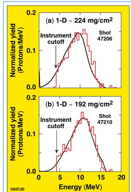
Figure 2. (a) The average secondary proton spectrum from shot 47206 (red) compares favorably with the spectrum (black) predicted by weighting the 1-D areal density profile by the experimentally measured temporal burn profile. (b) The same comparison as in (a) for shot 47210.
