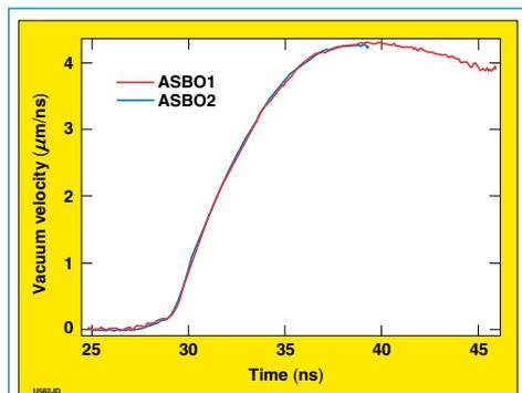
Figure 2. Comparison of velocities deduced from the two ASBO channels on shot 43369, an experiment on a thinner aluminum sample than that of shot 43384; the compression begins at 29 ns. The excellent agreement between channels is indicative of the stability and accuracy of this new system.
