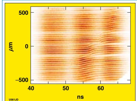
Figure 1. Image of VISAR data from upgraded ASBO system on shot 43384, an isentropic compression experiment on an aluminum sample having four steps (horizontal bands). The fringe position is proportional to the velocity of the rear surface. The thinnest step (bottom band) first signals the compression at 54 ns, the other steps show the arrival of the wave at successively later times.
