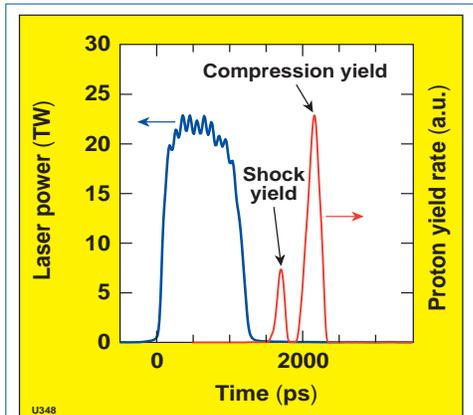
Figure 2. PTD record (red) obtained on an OMEGA implosion of a D<sup>3</sup>He-filled target displayed along with the laser pulse history (blue).
