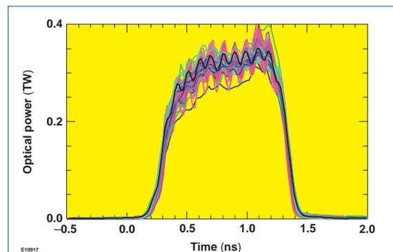
Figure 3. The streak camera recordings of all 60 beams of OMEGA overlaid for shot 23141. This was the first OMEGA 60-beam shot with all UV streak cameras active and calibrated. The 10-GHz modulation from the SSD system can be easily resolved.
