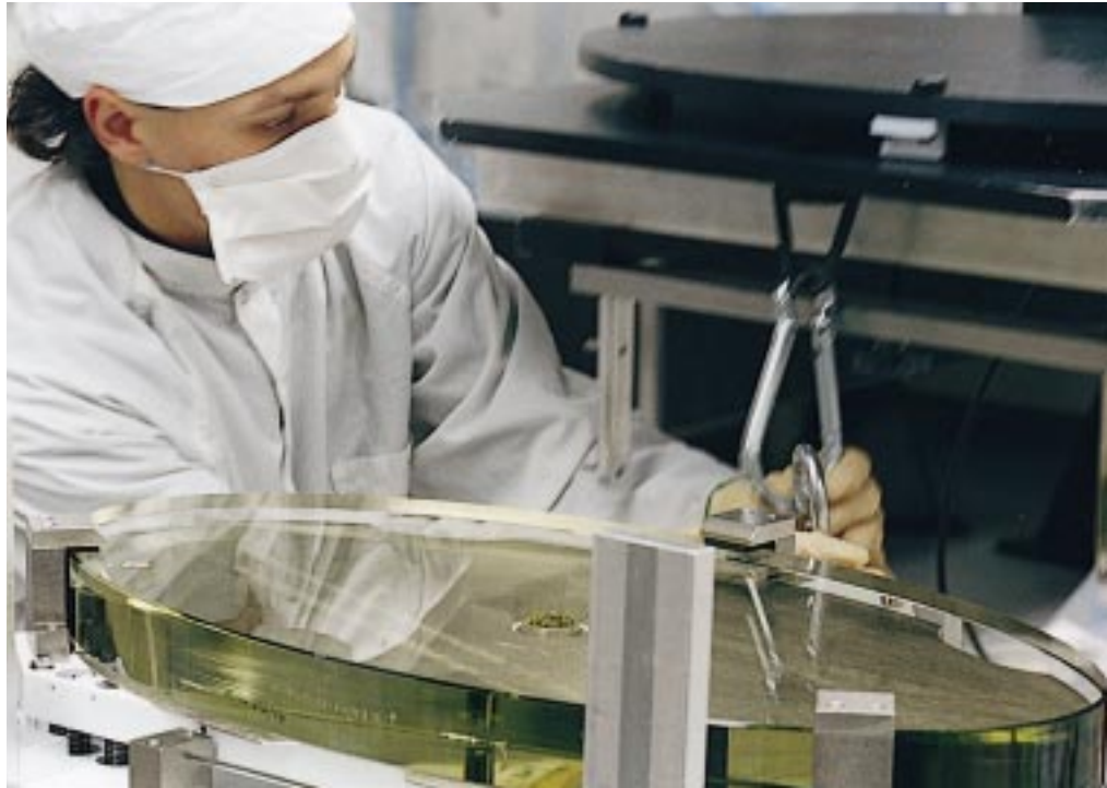
An OMEGA transport mirror coated with a 351-nm high reflector is shown being prepared for final testing.
